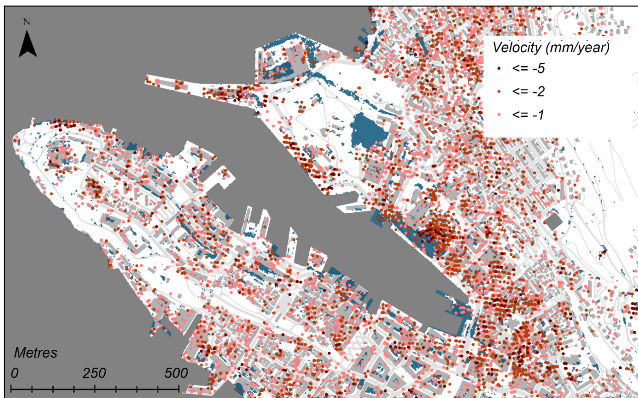
Figure: Areas of subsidence and flooding in Bergen city centre, Western Norway. The darker colour of the dot the higher average velocity (mm/year) for the subsidence. Blue color shows the flooded areas, with increasing water depth with darker colour (Venvik et al. submitted).
